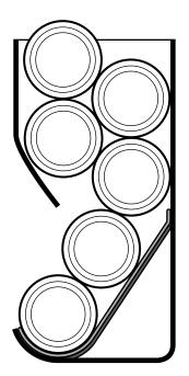
2. Load subsequent cans from the top ensuring that the cans are not dropped from a height greater than 15cm. (Dropping cans may damage dispenser and cause soft drink to fizz up).
