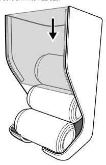
4. When removing cans pull the can up and towards yourself. Ensure that the can is not being pulled into the front lip of the dispenser.
