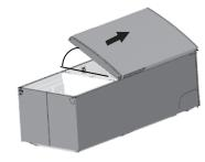
22. Replace LH centre hinge (kit content) by lifting the door slightly and sliding hinge into the door and placing the door down again.
