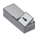
8. Unscrew 2 centre hinge screws. Remove the cover hole mullion with plastic lever.
