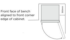
When positioned In a corner area, spacing of at least 350mm on the hinge side will allow the doors to open enough to enable the removal of bins and shelves.
