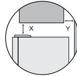
If you have a cupboard above the refrigerator with a rear gap of less than 100mm (Y), recommended minimum clearance at the top of the refrigerator increases from 50mm to 100mm (X).
