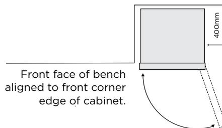
When positioned in a corner area, spacing of at least 400mm on the hinge side will allow the doors to open enough to enable the removal of bins and shelves.
