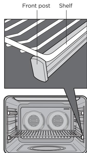
3. When fully inserted the shelf/tray should not interfere with the closed oven door.
