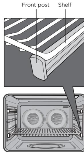
3. When fully inserted the shelf/tray should not interfere with the closed oven door.
