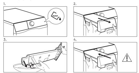
You can use the water from the water container as an alternative to distilled water (e.g. for steam ironing). Before you use the water, remove dirt residues with a filter.
