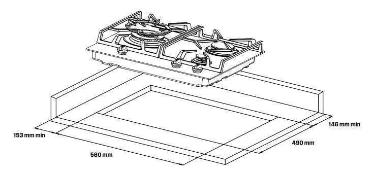
NOTE: Distances shown to adjacent walls/surfaces are for the distance to a combustible surface. If the surface is not combustible the measurement can be smaller than that shown.
