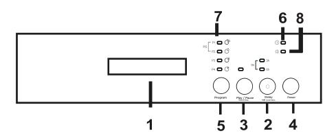
By pressing On/Off button(4), power on the machine. On/Off lamp lights as long as the machine is on. Select the suitable program by pressing Program button(5).
