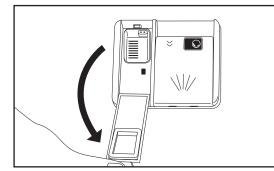
Fill the compartment with rinse aid until MAX level and then close the cap.
